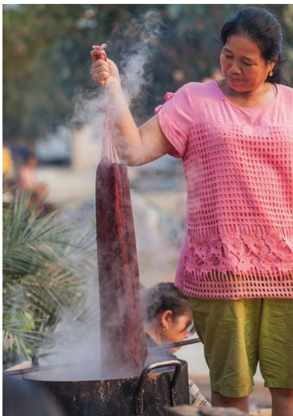
Skeins of silk have taken on deep, color-fast shades of red after less than an hour in the dye bath.
