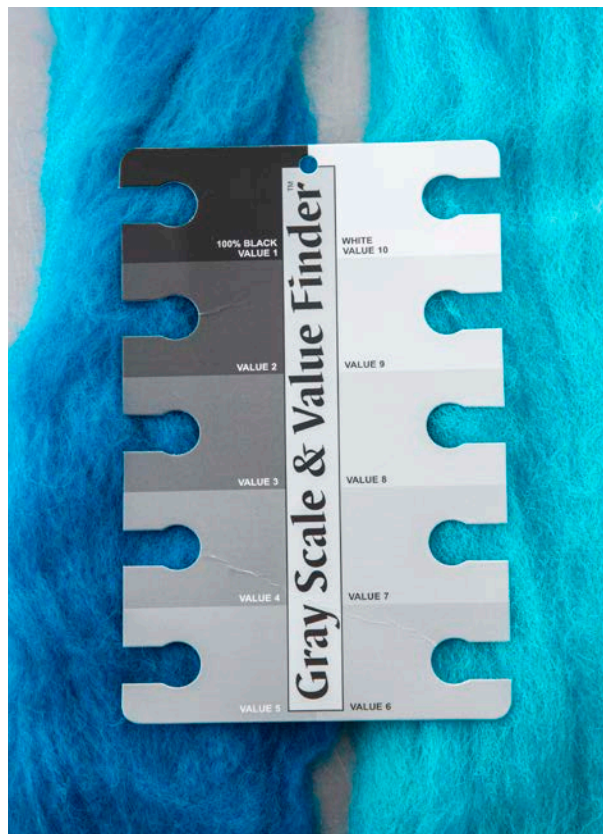
A gray-scale card can help you describe the value of colors. Here, where 1 is black and 10 is white, the darker fiber on the left is a value 2 and the lighter fiber is a value 7.
